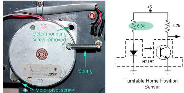
It was also found that the bridge track positioning would sometimes vary from power cycle to power cycle. Investigation and testing revealed that the home position sensor LED was being over driven. The 1k ohm current limiting resistor was changed to a 6.8k ohm resistor. The lower LED light intensity results in a consistent and repeatable home position.
