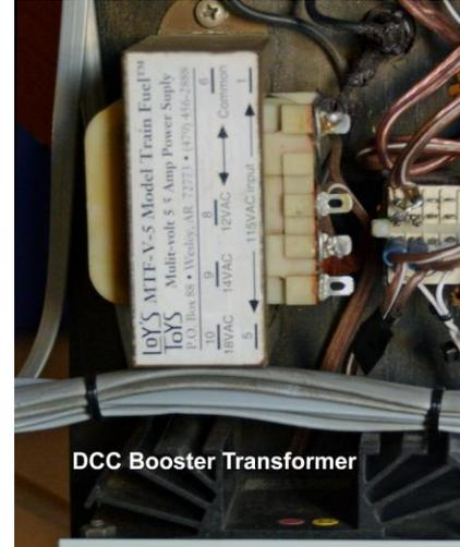
Figure 7: DB150 Booster Transformer
