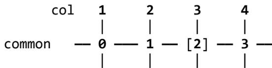
The keypad button columns are connected to a MCP23017 port. These pins are configured as input with pull-up. The keypad common is connected to ground. With no button pressed, all button coordinates will read high (1) due to the pull-up. A pressed button will read low (0). For multiple pressed buttons, the first button detected is used.
