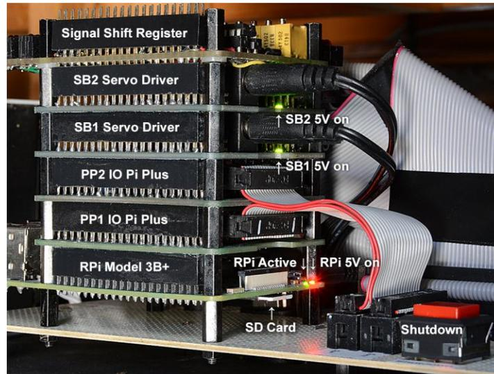
Figure 10: RPi Electronics Circuit Boards
