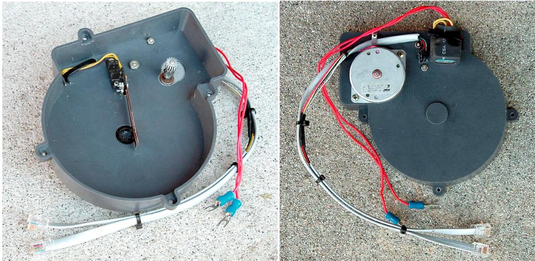
The bridge power wipers must be repositioned so as not to interfere with the home position sensor flag. The plastic piece that the wipers are attached to can be trimmed to clear the bridge gear spokes and attached to the home position sensor with epoxy. The wipers will need to be shortened a bit also. There is some flexing of the wipers which is why the sensor should be bolted to the base. The wires from the wipers exit through the original wiper mounting slot.
