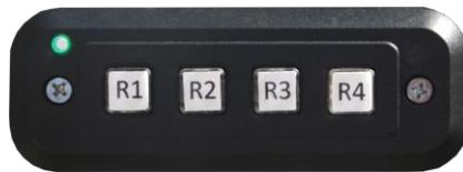
Figure 11: Holdover Turnout Positioning Buttons
