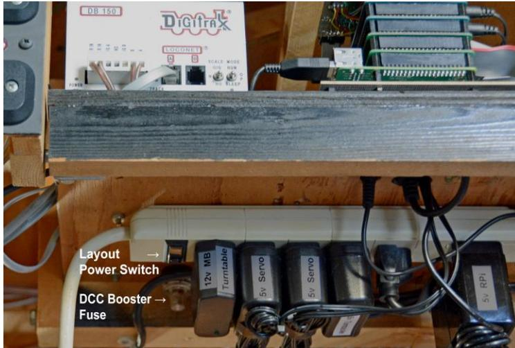
Figure 6: RPi Electronics Power Supplies
