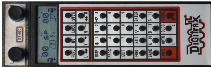
Figure 15: Digitrax DT400 Dual Throttle
