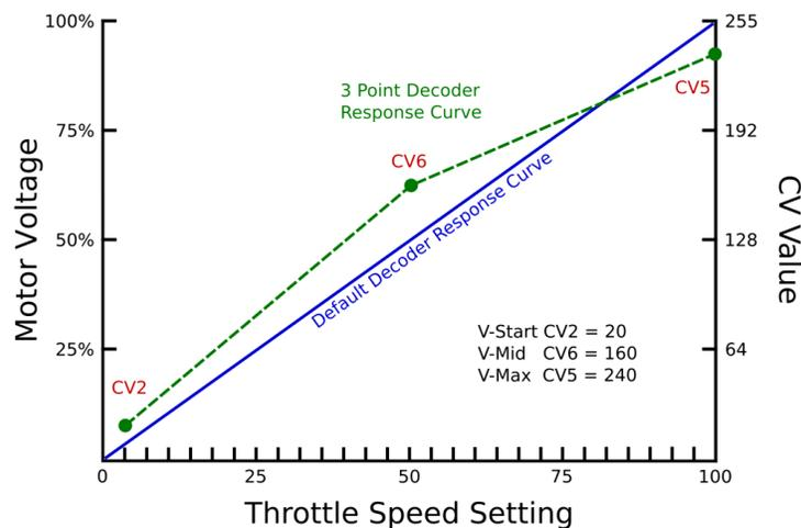
Figure 16: DCC Throttle Response Curve
