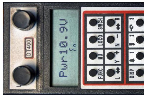
Figure 9: DCC DT400 Throttle Battery Power
