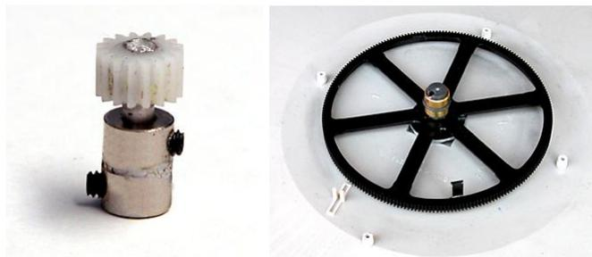
The D&B model railroad prototype turntable uses the final gear from the Walthers turntable drive motor assembly. This yields about a 12 to 1 ratio when driving the bridge gear in the Walthers Cornerstone Series (R) 90' turntable. The drive gear was drilled and epoxied to a short length of aluminum rod. Two wheel collars were soldered together and used to join the gear to the stepper motor shaft.
